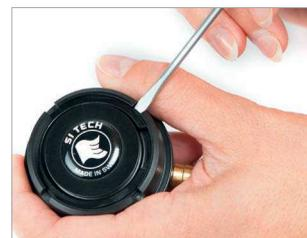
Use a small screwdriver to carefully remove the Locking Ring. Press towards the center of the lid to release it from the groove, then slightly press upwards.
