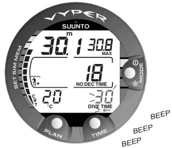
Fig. 3.32 Preset dive time alarm is activated.
