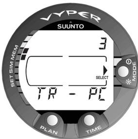
Fig. 4.15 Data Transfer Mode. [3 TR-PC].
