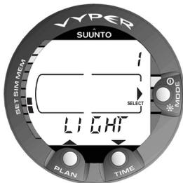
Fig. 4.41 Backlight Setting Mode. [1 LIGHT].
