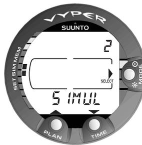
Fig. 4.3 Simulation option. [2 SIMUL].
