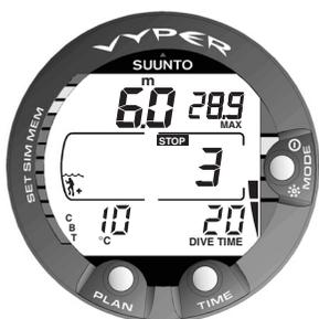
Fig. 3.10 Ascent rate indicator. Two segments.
