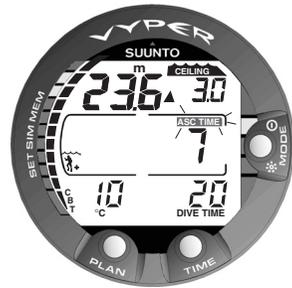
Fig. 3.16 Decompression dive, below the floor. The upward pointing arrow and the blinking ASC TIME label tell you to ascend. The minimum total ascent time including the safety stop is 7 minutes. The ceiling is at 3 m [10 ft].
