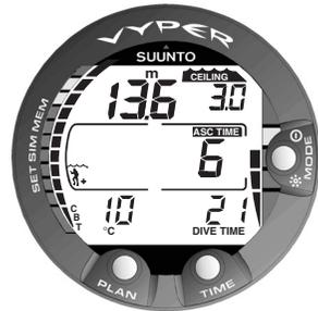
Fig. 3.17 Decompression dive, above the floor. The upward pointing arrow has disappeared and the ASC TIME label has stopped blinking, which means that you are in the decompression range.
