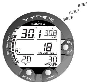
Fig. 3.33 Preset maximum depth alarm is activated.
