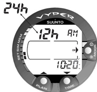
Fig. 4.35 Adjusting the Time.
