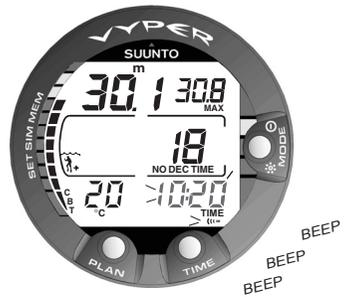
Fig. 3.31 Preset time alarm is activated.
