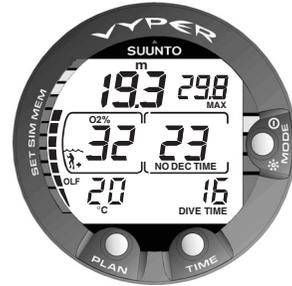
Fig. 3.22 Diving in the NITROX Mode. The O<sub>2</sub>% is set to 32%.
