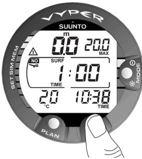
Fig 3.28 Surface interval, Surface time display. Pressing the TIME button will show the surface time display.
