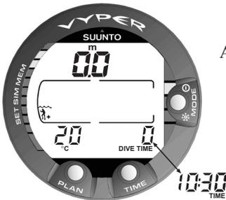
Fig. 3.4 Startup IV. The Surface Mode: The depth and dive time are zeros (as no dives have yet been made), and the temperature is 20°C [68°F].
