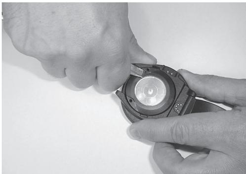
**Fig. 5.2 Opening of the securing ring.**
