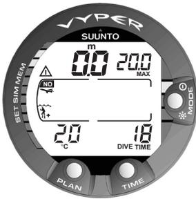
Fig. 3.27 Surface display. You have surfaced from a 18 minute dive, which maximum depth was 20.0 m [66 ft]. The present depth is 0.0 m [0 ft]. The airplane symbol indicates that you should not fly and the dive attention symbol indicates that you should prolong your surface interval time.
