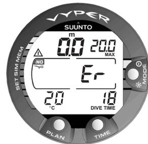
Fig. 3.30 Surface Mode after a violated decompression dive. The Er symbol indicates that you have violated the ceiling for more than three minutes. You must not dive again for at least 48 hours.
