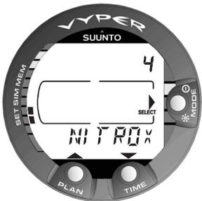
**Fig. 4.31 Nitrox/Oxygen Setting Mode.** [4 NITROX].
