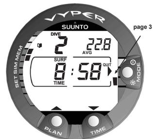
Fig. 4.9 Logbook, page III. The surface interval time and average depth.
