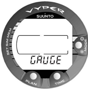
Fig. 3.3 Startup III. The Gauge Mode.
