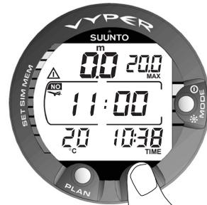
Fig. 3.29 Surface interval, no-flying time. Pressing the TIME button twice will show the no-flying time, indicated by an airplane symbol.
