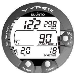
Fig. 3.11 Ascent rate indicator. Three segments.
