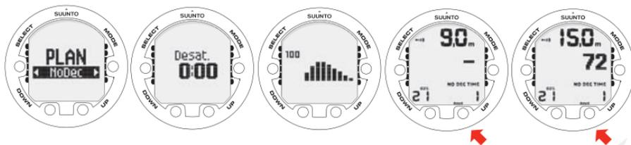
WHEN ENTERING THE PLANNODEC MODE THE DISPLAY FIRST BRIEFLY SHOWS TISSUE LOADING, THE REMAINING DESATURATION TIME BEFORE GOING INTO PLAN MODE. USE UP AND DOWN BUTTONS TO SCROLL DIFFERENT NO-DECOMPRESSION LIMITS. NO-DECOMPRESSION LIMITS LONGER THAN 99 MINUTES ARE DISPLAYED AS "--".
