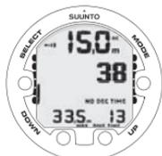
DIVE DISPLAY - PRESENT DEPTH IS 15 M, NO-DECOMPRESSION STOP TIME LIMIT IS 38 MIN. ELAPSED DIVE TIME IS 13 MIN.
