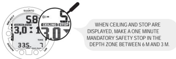
You must not ascend shallower than 3 m/10 ft with the Mandatory Safety Stop warning on. If you ascend above the Mandatory Safety Stop ceiling, a downward pointing arrow will appear and a continuous beeping starts. You should immediately descend to, or below, the Mandatory Safety Stop ceiling depth. If you correct this situation at any time during the dive, there are no effects on the decompression calculations for future dives.
