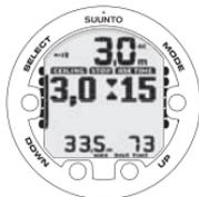
TWO ARROWS POINT AT EACH OTHER "HOUR GLASS": YOU ARE IN THE OPTIMUM CEILING ZONE AT 3 M. AND YOUR MINIMUM ASCENT TIME IS 15 MINUTES.
