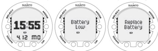
If the battery symbol is displayed in the Surface mode, or if the display is faded or weak, the battery may be too low to operate the dive computer, and battery replacement is recommended.
