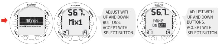
**NOTE** *If MIX2 is set ON, settings for all mixes are stored until changed. If MIX2 has an oxygen content of 22% or greater, settings for all mixes are stored until changed.*
