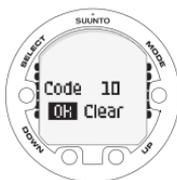
ADJUST WITH UP AND DOWN BUTTONS. ACCEPT WITH SELECT BUTTON.
