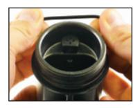
4) Apply a small amount of silicone lube on your finger tip and wipe it around the O-rings. Wipe off excess lubricant. The o-ring surface should have shiny, wet appearance.
