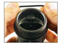
4) Apply a small amount of silicone lube on your finger tip and wipe it around the O-rings. Wipe off excess lubricant. The o-ring surface should have shiny, wet appearance.
