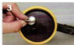
3 Lock the screw tight with a coin after charging.
